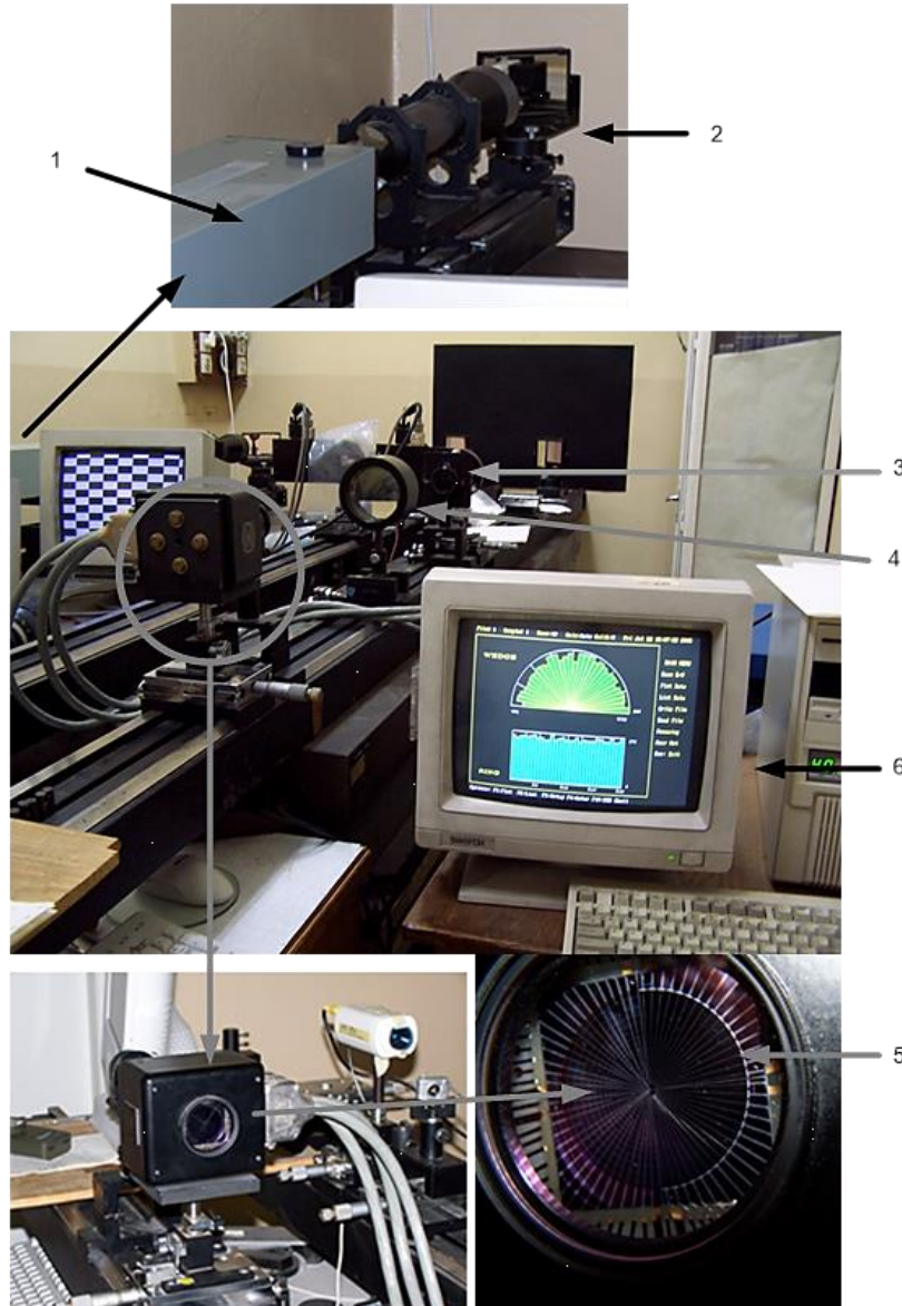
Fig. 4. Laboratory stand for images recognition in the diffraction plane, 1 - laser, 2 - collimator, 3 - spatial modulator, 4 - lens, 5 - ring-wedge detector, 6 - computer as a classifier in the artificial neural network
