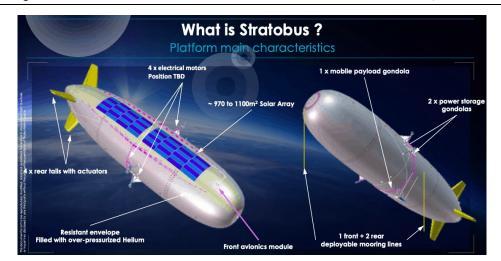
Fig. 7. Stratobus main characteristics [17]
