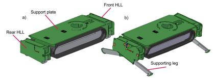
Fig. 6. Built-up tracked undercarriage : a) folded support legs, b) extended support legs [15]
