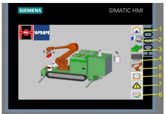
Fig. 12. Start screen of the operator control panel: 1 – home screen, 2 – hydraulic power supply screen, 3 – construction materials feeder screen, 4 – track undercarriage drive screen, 5 – robot screen, 6 – technology process procedure screen, 7 – failure screen, 8 – failure reset button [16]
