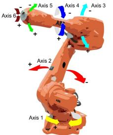
Fig. 3. ABB IRB 4600-40/2.55 robot axis
