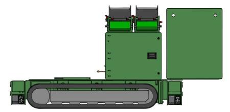
Fig. 9. Control cabinet mounted on the tracked undercarriage [15]
