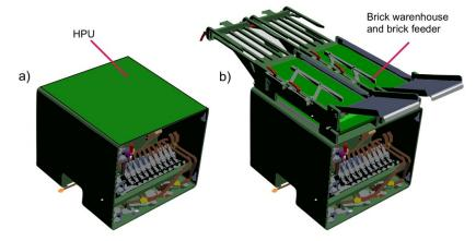
Fig. 7. Design elements: a) hydraulic power unit (HPU), b) hydraulic power unit and brick warehouse with a brick feeder [15]
