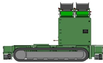
Fig. 8. Hydraulic power unit and brick warehouse with a brick feeder mounted on the tracked undercarriage [15]
