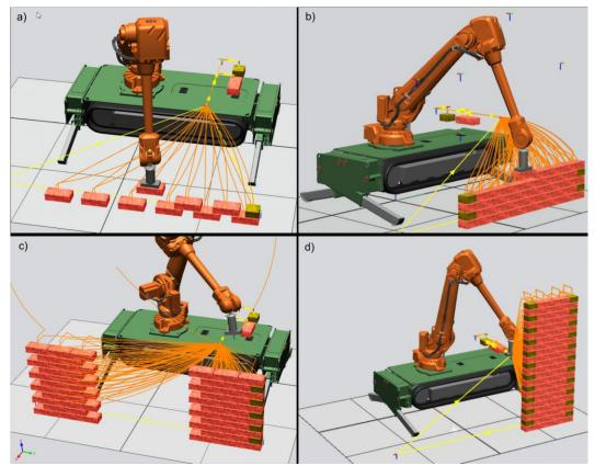
Fig. 2. Visualization of the bricklaying process in ABB RobotStudio: a) hit and miss brickwork, b) stretcher bond, horizontal wall, c) stretcher bond, hole in a wall, d) stretcher bond, vertical wall [15]
