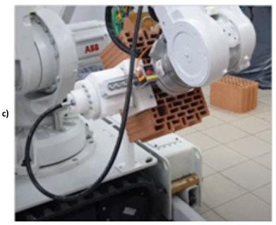
Fig. 14.c View of the bricklaying process on a partition wall: apply mortar to the bricks  $\left[ 16 \right]$
