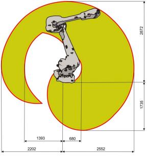
Fig. 4. Dimensions of the workspace of the ABB IRB 4600-40/2.55 robot in mm
