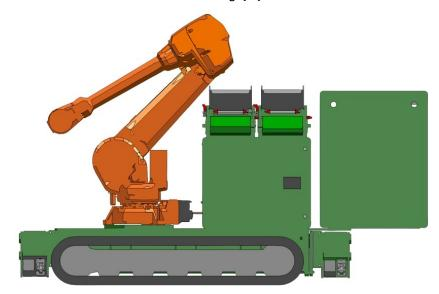
Fig. 10. ABB Robot mounted on the tracked undercarriage [15]
