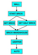
Fig. 13. Flow chart of the technological process procedure in manual programming mode
