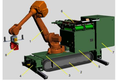
Fig. 1. 3D model of mobile ZSM: 1 – ABB industrial robot, 2 – Hinowa tracked undercarriage, 3 – base, 4 – hydraulic lifting and leveling module, 5 – hydraulic control unit, 6 – brick warehouse with a brick feeder, 7 – control cabinet with an operator panel, 8 – hydraulic gripper [15]
