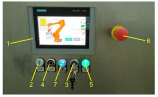
Fig. 11. View of the control elements in the control cabinet: 1 – HMI operator panel, 2 – automatic control cycle start button, 3 – control mode switch, 4 – automatic cycle STOP button, 5 – control cycle indicator light, 6 – emergency STOP button, 7 – emergency STOP reset button [16]
